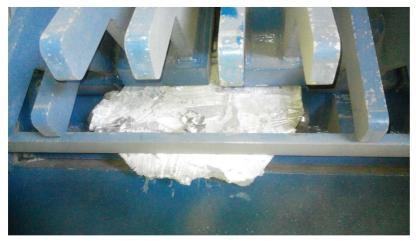
Fig. 3: ejected 10 kg chunk of aluminium
