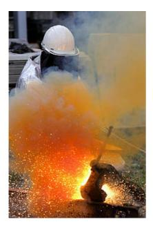
Gas-cutting with fuel gas as propane or acetylene and oxygen is generally used for breaking down large machines or other bulky pieces of scrap. These processes are generating large amounts of smoke and dust containing iron and iron oxide fines and hydrocarbon compounds, causing large yellow/ocher coloured clouds of dust.
