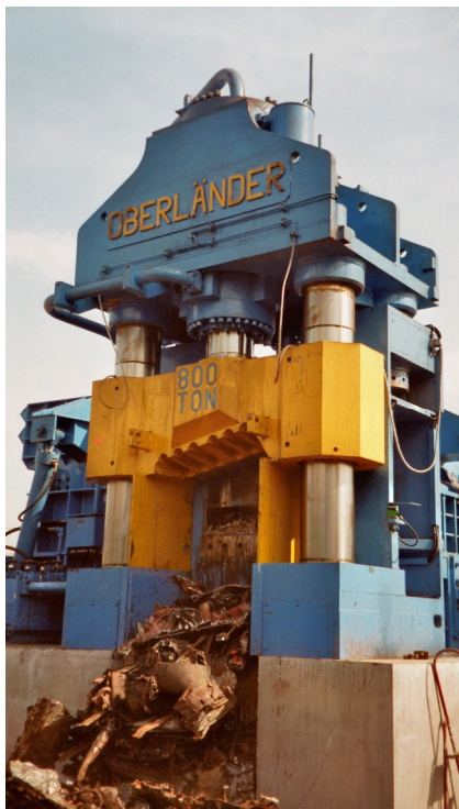
Pic.: The distinctive column design of the Oberländer shears
