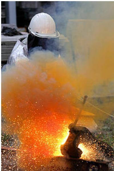
Flame-cutting with fuel gas as propane/methane and oxygen is generally used for cutting down large machine structures or other bulky pieces of non-shearable scrap. These processes are generating large amounts of smoke and dust.
