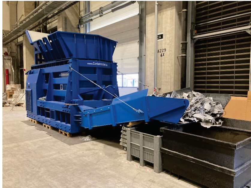
Pic. 2: Complete press-shear installation with discharge chute
