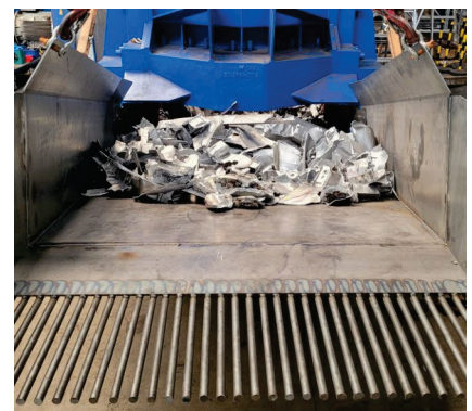
Pic. 3: Press-shear discharge with finger screen
